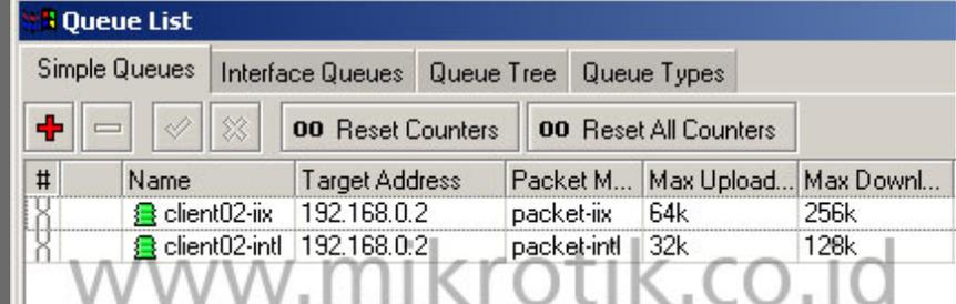
The screenshot shows the Mikrotik WinBox interface for the Queue List. It features a navigation bar with tabs for Simple Queues, Interface Queues, Queue Tree, and Queue Types. Below the tabs are control buttons for adding, deleting, and refreshing queues, along with 'Reset Counters' and 'Reset All Counters' buttons. A table displays the configured queues with columns for ID, Name, Target Address, Packet Mark, Max Upload, and Max Download.
